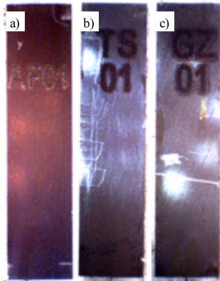
Figure 23: Optical images of FeCrAl specimens after peak irradiation fluence of 1.21 \times 10^{21} n/cm 2 ( E > 0.1 MeV – dpa was not reported) in PWR-like water conditions; (a) Kanthal AF, (b) C36M3, and (c) C06M. Images courtesy of Y. Katoh (ORNL).
